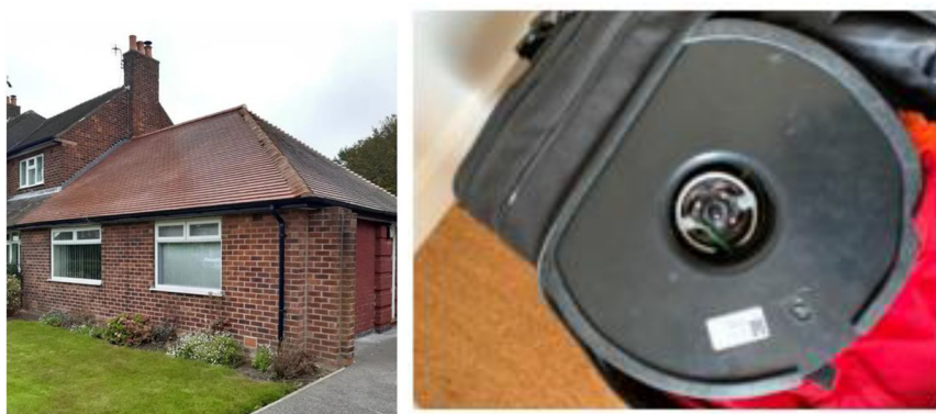
Figure 13. (L-R) retrofitted building: a very low min fan is required for the fan tests, with a large restrictor plate fitted
