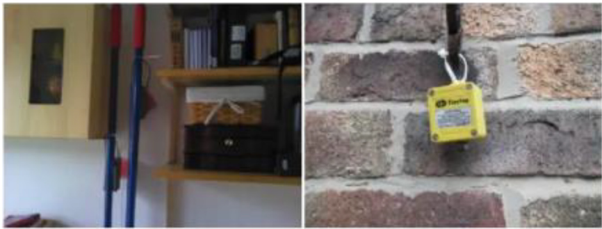
Figure 8. The apparatus set up in an occupied home (left-hand image), with clamps and teleports (blue poles) supporting the heat flux plates (red discs) and indoor temperature sensors
