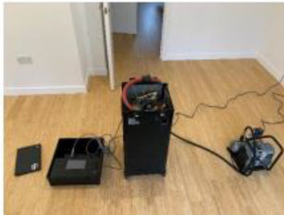
Figure 11. (L-R) Complete 40 L pulse set-up used in this configuration for all text cases; blower door fan mounted and sealed in a panel cut to the size of the window opening
