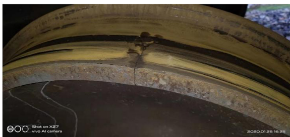
a rim crack of 28 mm
