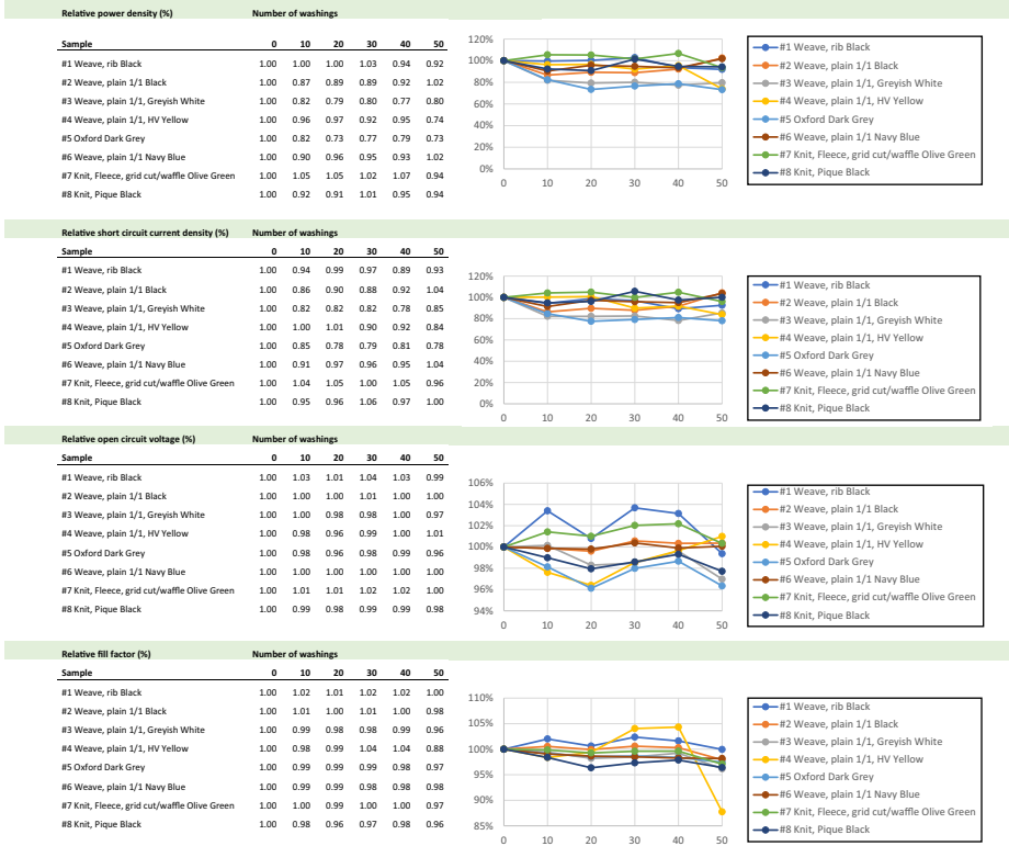
Notes: The same data is shown as a table and a graph. In the graph, the horizontal axis is the number of washing cycles and the vertical axis is the measured or calculated quantity corresponding to the table
