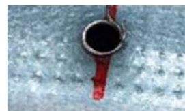
Pull-out bending failure from the experiment (4075 Batten and 12g-24 Tek) Sivapathasundaram et al. (2018)
