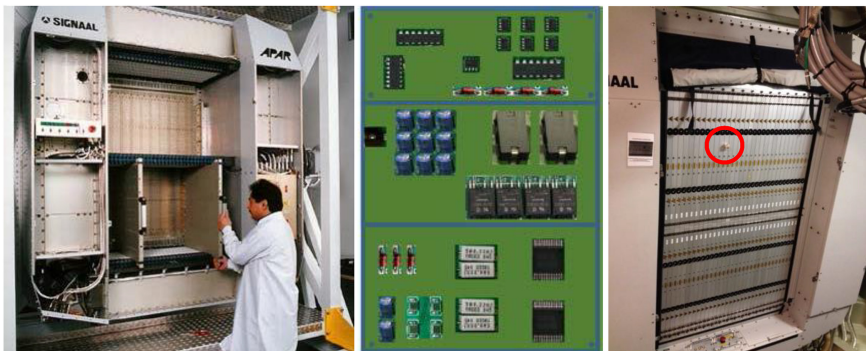
Figure 5. Left: taking out a column assembly (CA) from the radar; middle: generic layout of the PCB; right: vibration sensor (in red circle) positioned on CA (Politis, 2015; Tinga et al., 2017)
