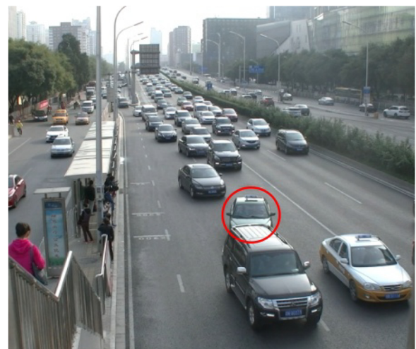
Figure 7 Non-standard lane change vehicles in the weaving area
