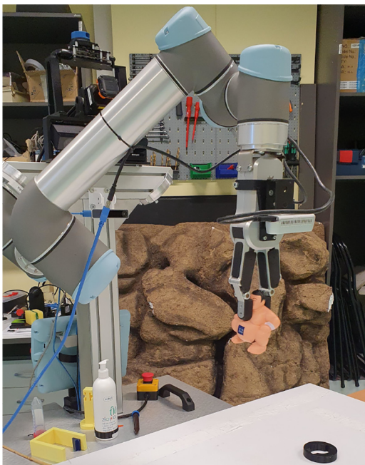
Figure 1 Robot collecting objects using CNN for object detection and grasping
