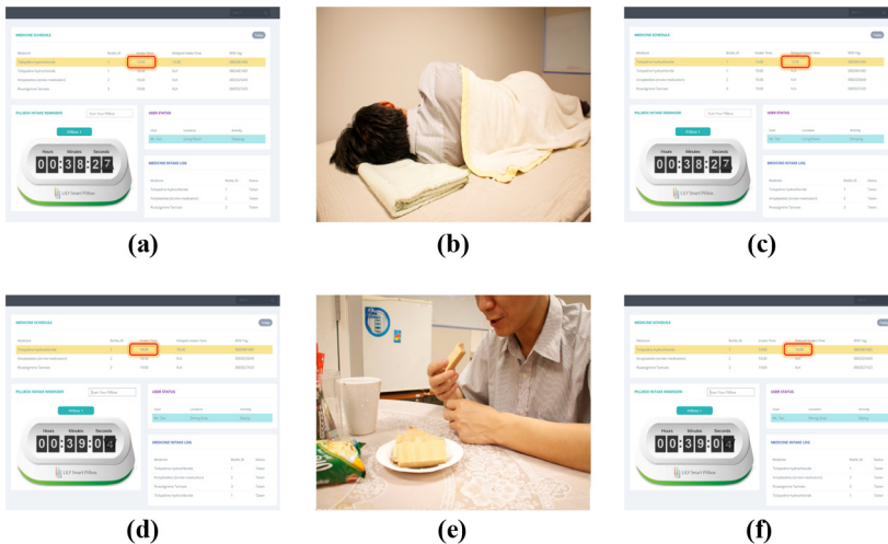
Notes (a) Reminder for Ticlopidine Hydrochloride was scheduled at 13:00; (b) context recognized by the system: user is sleeping; (c) reminder for Ticlopidine Hydrochloride is delayed to 13:30; (d) reminder for Ticlopidine Hydrochloride was scheduled at 18:00; (e) context recognized by the system: user is eating; (f) reminder for Ticlopidine Hydrochloride is delayed to 18:30
