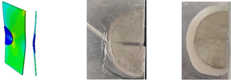
Cracked Specimen with Semicircular patch ( $R_p = 17\text{mm}$ )
