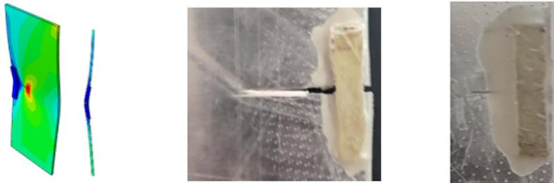
Cracked Specimen with Rectangular patch, ( $w_p = 5\text{mm}$ ) at position, ( $x = 0$ )
