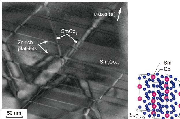
**Figure 1.** Bright-field TEM image of the Sm-Co magnets containing nanoscopic  $\text{SmCo}_5$ ,  $\text{Sm}_2\text{Co}_{17}$  and Zr-rich phases
