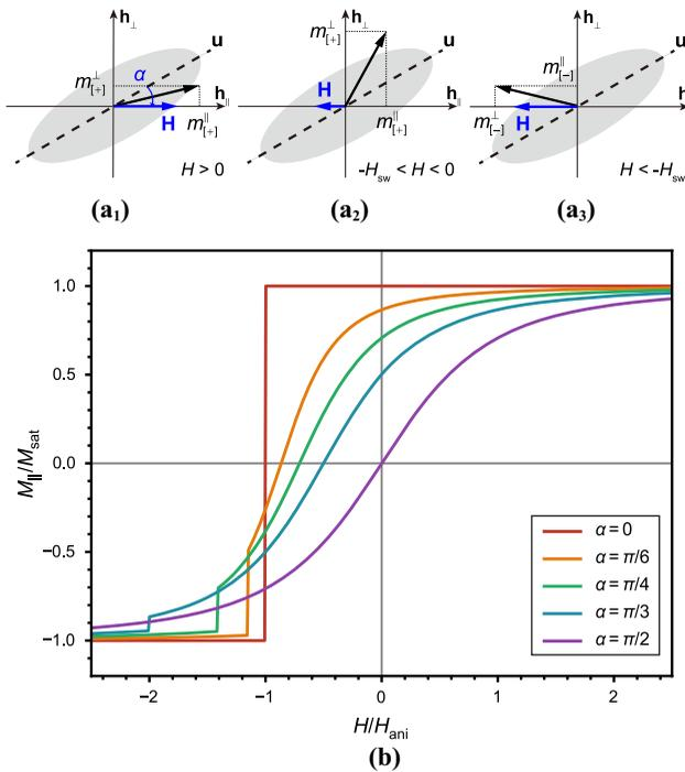
**Notes:** (a<sub>1</sub>)  $H > 0$ ; (a<sub>2</sub>)  $-H_{sw} < H < 0$ ; (a<sub>3</sub>)  $H < -H_{sw}$ .  $m_{[+]}^{\parallel}$  and  $m_{[-]}^{\perp}$  and are, respectively, the longitudinal and transverse magnetization components with [+ ] for the upper branch and [- ] for the lower branch.  $H = Hh_{\parallel}$ ; (b) Longitudinal half-cycle hysteresis of parameterized vector hysteron with different easy axis orientations
