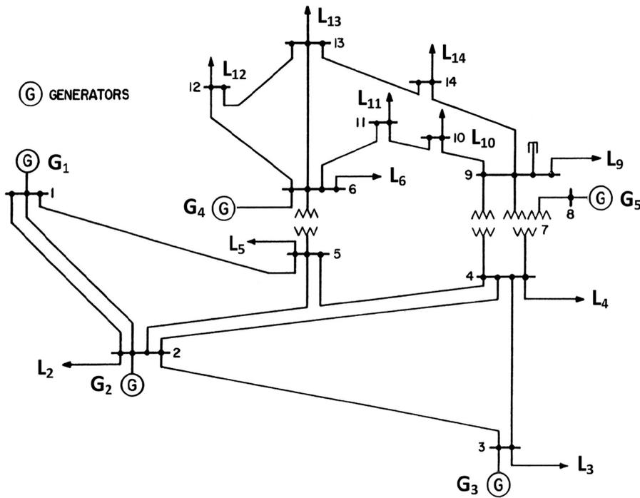
Figure 2. Single line diagram for IEEE 14 bus system.
