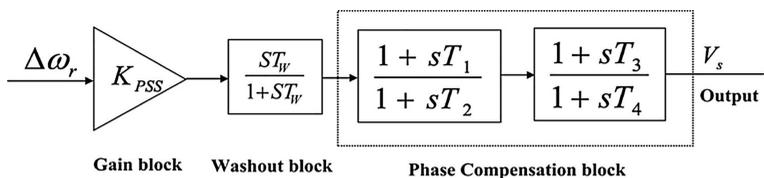
Figure 3. Block diagram of two staged PSS.
