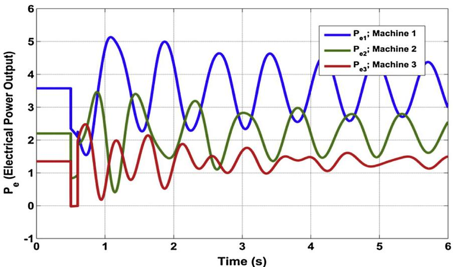
**Figure 9.** Electrical Output ( $P_e$ ) under heavy load when PSS is not installed (WSCC 3 machine 9 bus system).
