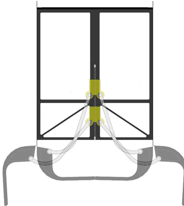
**Figure 10** Fuselage internal layout: left – original, right – redesigned
