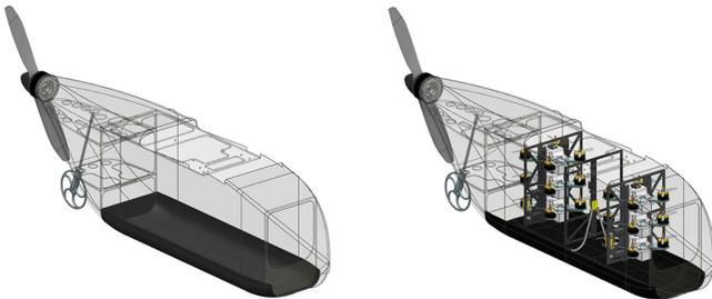
monocoque structure of this airframe section. The presence of the two drone-holding frames and the opening mechanism frame for the DB doors significantly increases stiffness of the whole structure.
